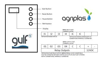
This unit only uses dry contact inputs.
