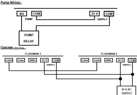
NOTE: Supply wires must be swopped on second FLUSHMAN (24V to COM & COM to 24v).
